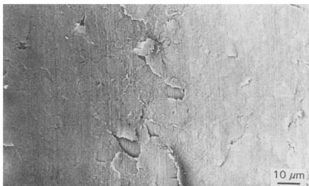
Figure 7 Thin layers of composite resins deposited on the wear track, which were generated by the diamond indenter with a 10 N applied load (scratching direction: top to bottom).
